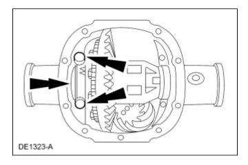
4. Install the original differential bearing shim on the RH side.
