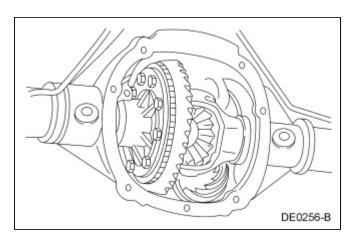
2. Install the originally removed differential bearing shim on the LH side.
