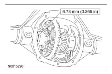
3. **NOTE:** Apply pressure toward the LH side to make sure the LH differential bearing cap is seated.
