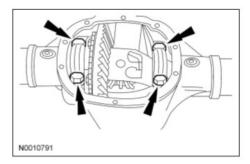
3. **NOTE:** Place a wood block between the pry bar and the axle housing to protect the machined surface from damage.
